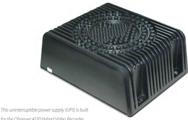
for the Observer 4120 Hybrid Video Recorder (HVR). Voltage spikes and drops are leveled out to create a steady and clean electrical current to the HVR, protecting valuable storage devices from corruption in harsh mobile environments. In the event of complete power loss, the UPS allows the HVR to gracefully shut down, protecting recorded video and data integrity.
