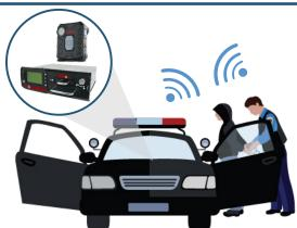
As soon as the officer is back within the Wi-Fi range, video from the Prima Elite body camera is automatically uploaded to the ICOP PRO system. Body camera recordings are then synchronized with the matching incar recordings.
