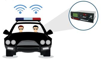
Once you're logged in, the ICOP PRO HD in-car system and the Prima Elite body camera automatically synchronize together over Wi-Fi. The ICOP PRO HD records video from each of the mobile cameras and stores it onto the hard drive until video is ready to be wirelessly downloaded back at the station.
