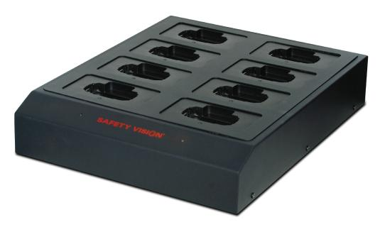
The 8-bay docking station offers agencies fast and efficient operation by simultaneously charging and uploading files from up to eight SV-BodyCam units – all at the same time. Complete with two high-speed USB 3.0 interfaces for quick transfer rates, simply dock the body cameras and the 8-bay docking station automatically uploads all recorded files to the connected PC or FTP server. Once data is fully imported, all recorded files are then automatically deleted from each body camera.
