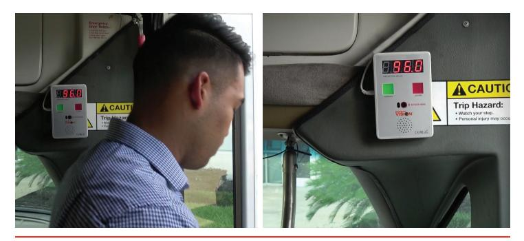
Using a high-precision temperature measurement sensor imported from Belgium, Safety Vision's IR thermometer measures the human body surface temperature without any contact. When an abnormal body temperature is detected, an audible voice warning will occur. This can be used as a stand-alone product or integrate with walk-through metal detectors, doors, intelligent access control systems, and more.
