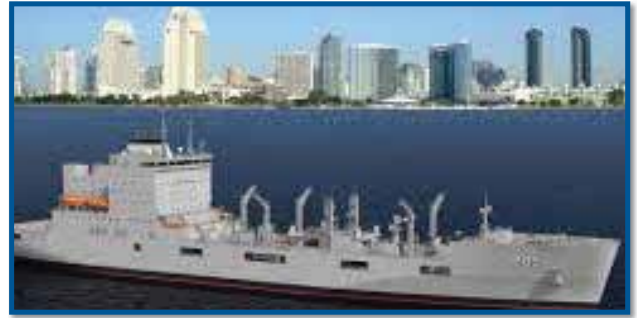
The John Lewis-class ships are based on commercial design standards and will recapitalize the current T-AO 187 Class Fleet Replenishment Oilers to provide underway replenishment of fuel to U.S. Navy ships at sea
